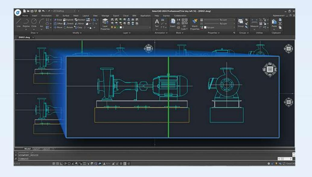
**VPMAX/VPMIN**: VPMAX allows you to expand the current layout viewports and switch to Model Space for editing without worrying about messing up viewports' scales and limits. VPMIN allows you to restore the current layout viewport.
